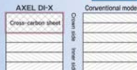
Cross-sectional image of carbon on the crown
